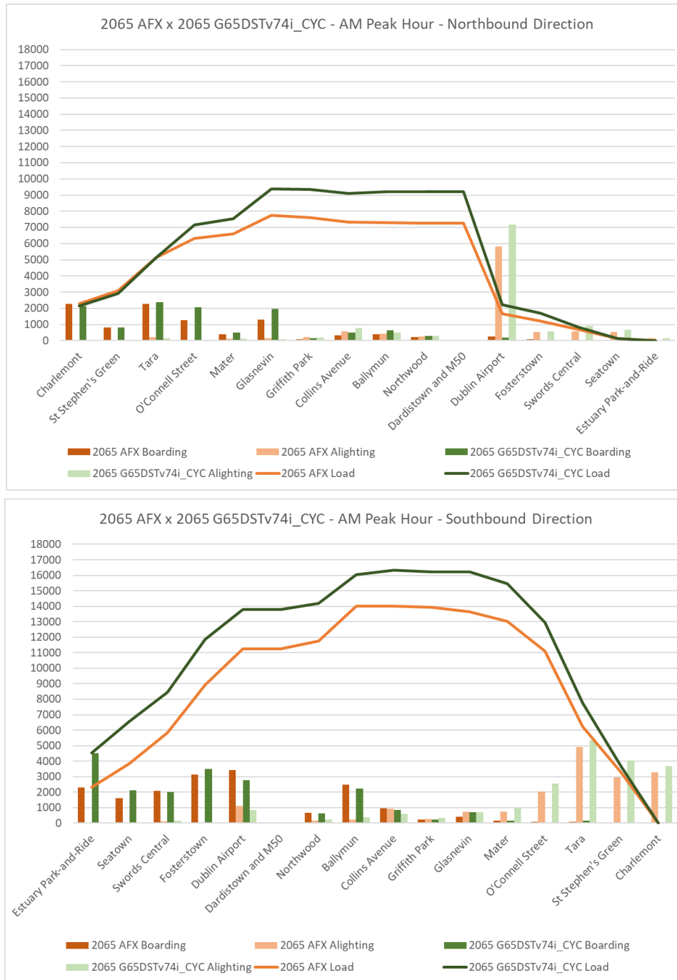
Figure 2—5: Metrolink - Line Flows - AM Peak - Prior GDA V New GDA (2065)
